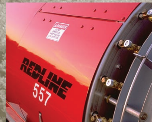
Positive "on" positive "off" double rollover drip-proof ceramic nozzles with diaphragm check valves ensure manifold stays full.
