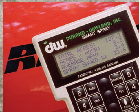
Cab-mounted SmartSpray controller gives up-to-the-second information on sprayer performance, including chemicals saved.
