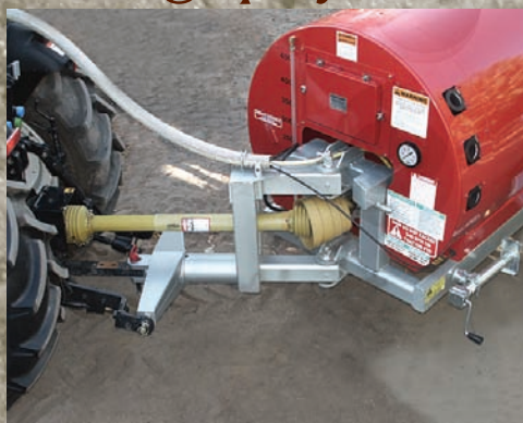
Rugged new "SureTrac" or conventional hitches available for both models. "SureTrac" connects to drawbar and 3-point hitch arms.
