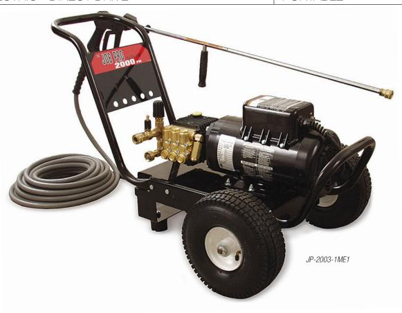
**Pump:** Direct drive triplex piston General or AR pump with ceramic plungers • Stainless-steel and brass unloader • Adjustable pressure • Forged brass manifold • Thermal relief valve • Safety relief valve • In-line water strainer • Adjustable low pressure detergent injection
